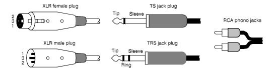
All input and output **XLR** connectors are 3 wire differentially balanced. These have 3 connector pins: Pin 1 = ground (screen), Pin 2 = signal hot (+), Pin 3 = signal cold (-).
