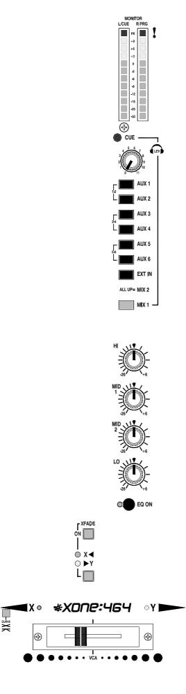
**Check the sound using the Cue system**. With the music playing press the large CUE switch. The switch itself and the master section CUE led light to show that the cue monitor is active. The channel signal is now sent to the headphones. Slowly turn up the headphones level control until you hear the music at comfortable volume.
