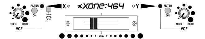
**FILTER ON** Each X and Y filter has its own ON switch. The blue led lights when the filter is switched on. The signal is not affected by the filter if the switch is in its off position. Use this to punch the filter effect in or out.
