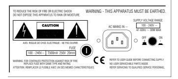
Read the **SAFETY INSTRUCTIONS** printed at the front of this User Guide. Check that the correct mains lead with moulded plug has been supplied with your console. The power supply accommodates mains voltages within the range 100-240V without changing any fuses or settings.
