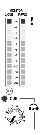
**MONITOR / MIX2 METERS** A pair of meter bars displays the level of the selected monitor source or CUE. With all selector switches up these default to display the post-fader left and right output levels of stereo Mix2. When SPLIT CUE is selected the left meter displays the active CUE signal, the right displays PRG (program), the switch bank source in mono.
