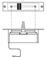
To replace either version of crossfader use a medium size cross-point (Pozidriv) screwdriver to undo and remove the two outer screws on the crossfader plate. Do not remove the inner screws.
