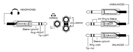
**LOCAL (BOOTH) MONITOR OUTPUTS** A pair of 3 pole TRS jack sockets provide left and right outputs from the console local monitor system. These are impedance balanced and can be connected to balanced or unbalanced equipment as shown above. Nominal operating level is –2dBu but gain is available to drive +4dBu if required. Independent control is provided for the local and the headphones monitor systems. This output typically feeds the DJ booth monitor with the music only mix, and Cue if required.
